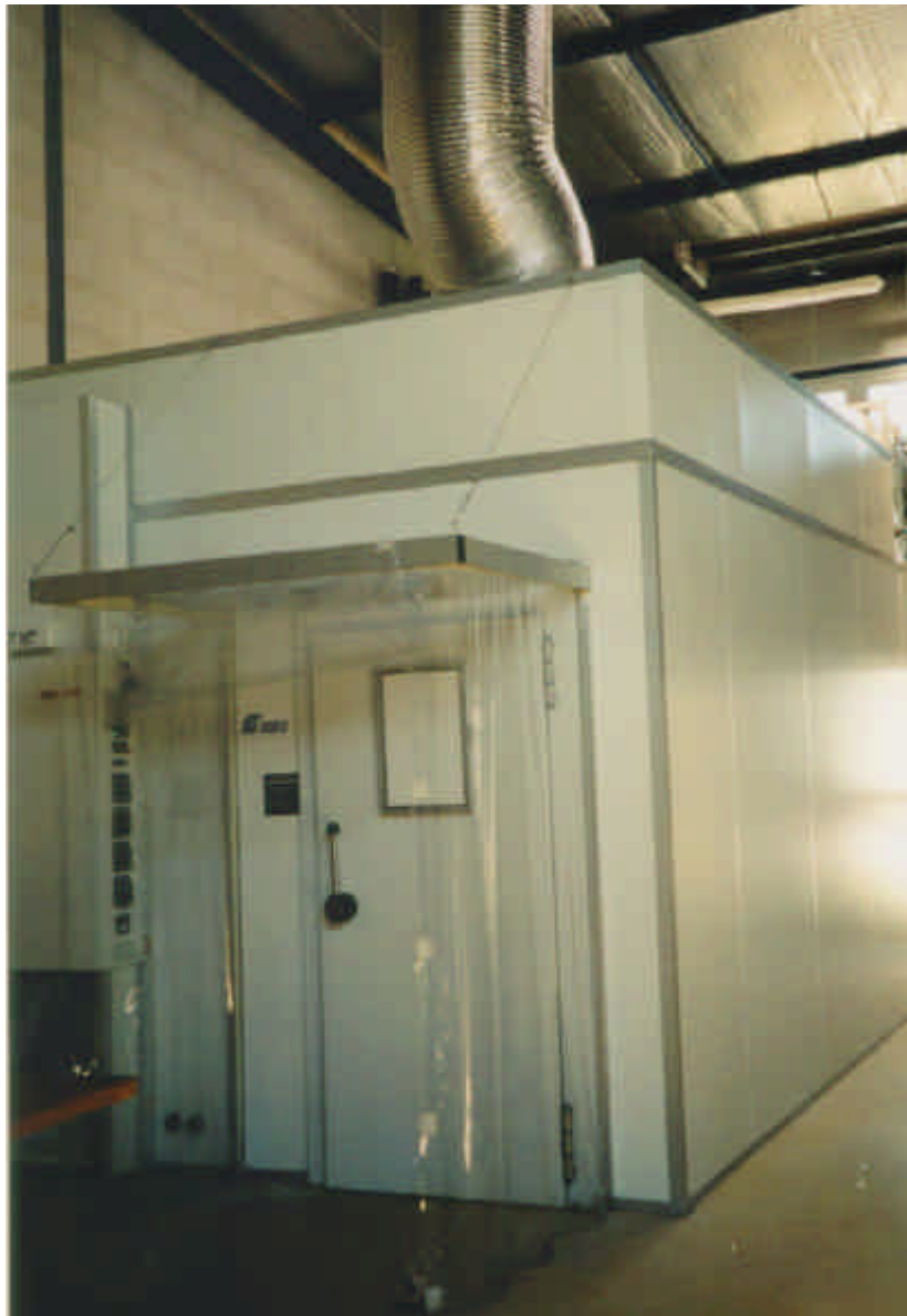
Figure 3-1: Phytotron external view (the hopper is open, the 180° swivelling door is close, left the electric commands)
