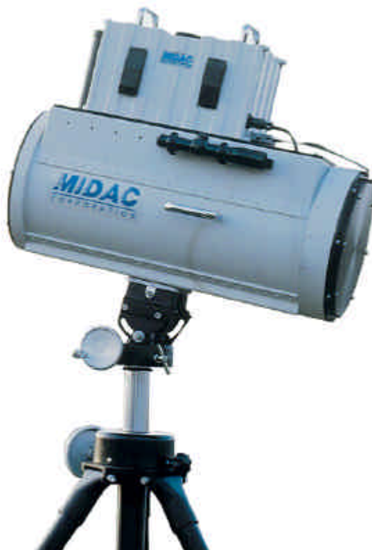
Figure 5-5: An example of spectroradiometer (Midac Air Monitoring). On top, the interferometer module, at the bottom, a telescope.( http://www.midac.com/ )
